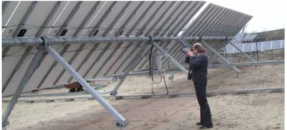
Volker Denzler, thermography expert at SOLON's after sales services department, takes thermal images from the back of a module to avoid reflections.
