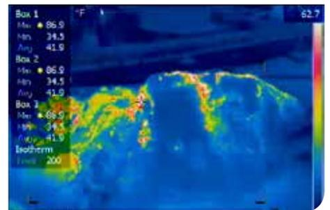
The FLIR A310f thermal imaging camera easily detects hot spots before they have time to cause dangerous fires.
