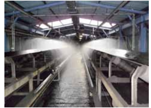
The PLC immediately stops the conveyor belt and activates the sprinkler system when the temperature alarm is triggered.
