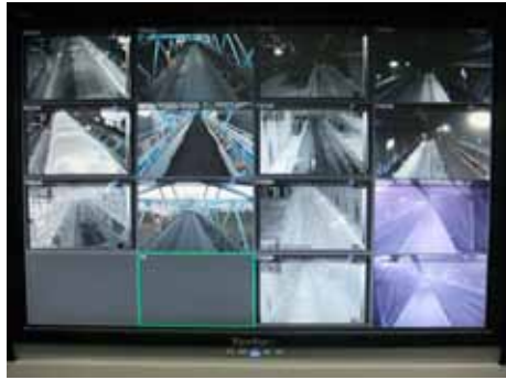
The footage and thermal data from the seven FLIR A310 thermal imaging cameras is sent to the PLC and to the control room.
