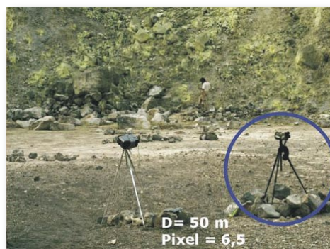
FLIR Systems cameras located along a NE-SW trending line, Vulcano Fossa fumarole field, Vulcano Island.
