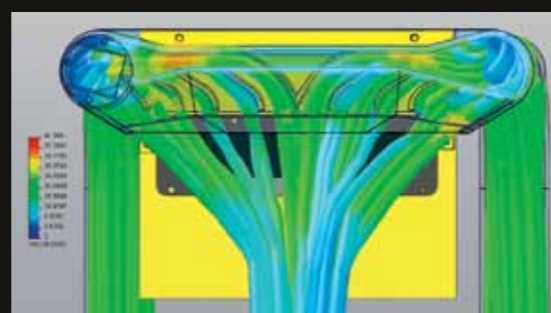
Air purge designed with Computational Fluid Dynamics
